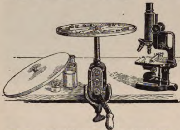
Fig. 178. Centrifuge and microscope for the study of bacteria.
